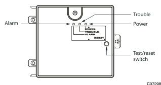
Fig. 26 - Controller Assembly
